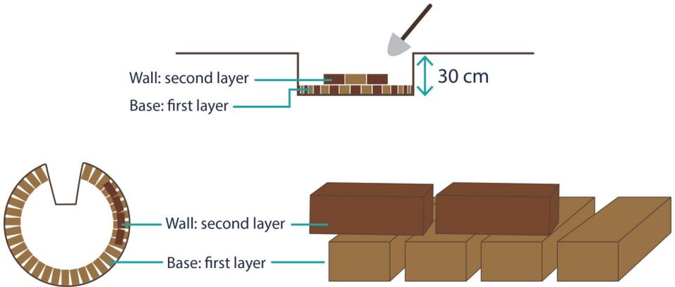
**Step 3:** We then started constructing the 1 metre wall structure of the KHG from foundation using the mixer of anthill soil and water to form a paste.
